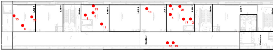
Fig. 3. WSN topology associated with the Heat dataset
